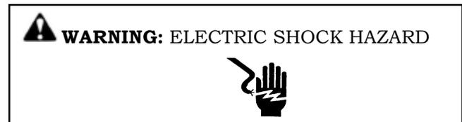
2. **ELECTRICAL:** Connect the machine to an electrically grounded circuit that is fuse or circuit breaker protected. Do not use any type of adapter. If the correct type of receptacle is not available, have one installed by a qualified electrician.
