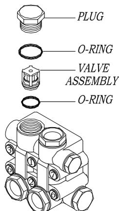
6. Malfunctioning valve assemblies must be replaced.
