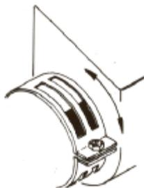
3. Tighten the cap screw retaining the air bands.
