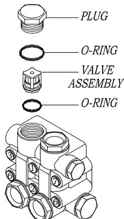
6. Malfunctioning valve assemblies must be replaced.
