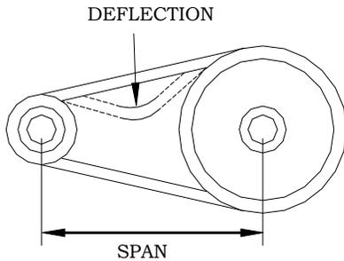
1. Correct belt tension will allow a 1/64-inch deflection for each inch of span between pulley centers with a 6-pound force applied in the middle of the span. EXAMPLE: A 6-pound force applied at the middle of an 8 inch span should produce a deflection of 8/64 inch or 1/8 inch.
