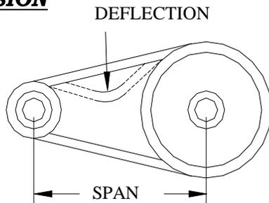
1. Deflection for each inch of span between pulley centers with a 6-pound force applied in the middle of the span. EXAMPLE: A 6-pound force applied at the middle of an 8 inch span should produce a deflection of 8/64 inch or 1/8 inch.
