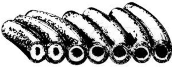
Above is a cross section view showing the progressive liming of coils.
