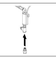
**STEP 2:** Connect high pressure hose from pressure washer (not included) to burner module.
