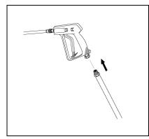
**STEP 4:** Attach high pressure wand to spray gun of connected pressure washer (Not Included).
