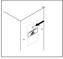
**STEP 6:** Turn on burner switch. Pilot ignition will begin to spark. Confirm pilot light ignition, if unsuccessful, turn off switch and turn on again. If pilot continues to spark, but not light, consult trouble-shooting guide.
