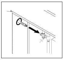
**STEP 3**: Connect high pressure hose from pressure washer when connecting to burner module outlet.
