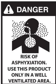
**DANGER:** Risk of asphyxiation. Do not inhale fumes. Use this product only in a well ventilated area. Running this product indoors can result in death due to carbon monoxide, a poisonous gas you cannot see or smell. Never operate indoors even if windows and doors are open. Only use outdoor and far away from windows, doors, and
