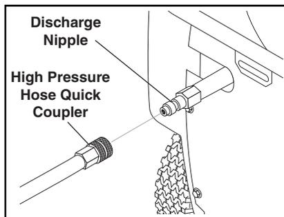
**STEP 2:** Connect the high pressure hose quick coupler to discharge nipple by sliding the quick coupler collar back and inserting quick coupler on to discharge nipple and pushing the quick coupler collar forward to secure it.
