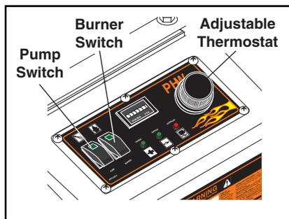
**STEP 4:** Press the pump switch "ON" and then pull the trigger on the spray gun to activate pressure switch which starts machine (For auto start machines only).
