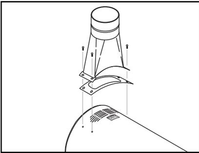
**STEP 4:** Adding exhaust vent pipe to your oil fired burner is not recommended because it restricts air flow. This causes carbon build-up, which affects the operation and increases maintenance on the coil. If a stack must be used, refrain from using 90° bends. If the pipe can not go straight up then use only 45° bends and go to the next larger size pipe. The overall pipe length must not exceed 6 feet in length. Air adjustments will be required after installation.
