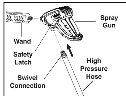
**STEP 3:** Attach wand to spray gun using teflon tape on threads to prevent leakage. Attach swivel connector on high pressure hose to spray gun using teflon tape on threads. Engage safety latch to prevent from triggering gun.
