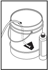
**STEP 1:** Use Landa detergent designed specifically for pressure washers. Household detergents could damage the pump. Prepare detergent solution as required by the manufacturer. Fill a container with pressure washer detergent. Place the filter end of detergent pick-up tube into the detergent container.
