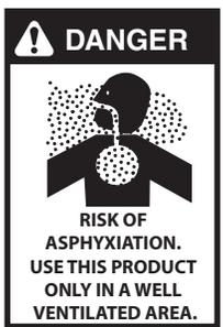
**DANGER:** Risk of asphyxiation. Use this product only in a well ventilated area. Running this product indoors can result in death due to carbon monoxide, a poisonous gas you cannot see or smell. Never operate indoors even if windows and doors are open.
