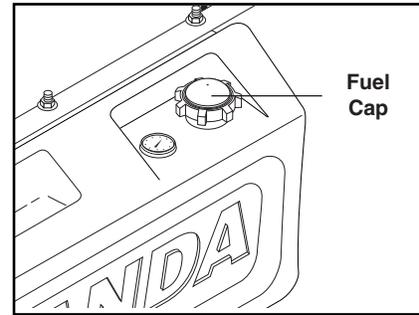
**STEP 3:** Fill fuel tank with proper fuel: kerosene, No. 1 home heating fuel or diesel.
