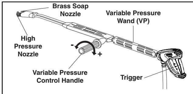
**STEP 5:** Selection of high or low pressure is accompanied by turning the handle. **Note:** High pressure nozzle must be inserted at end of wand to obtain high pressure. To apply soap, see Detergent and General Cleaning Techniques section.
