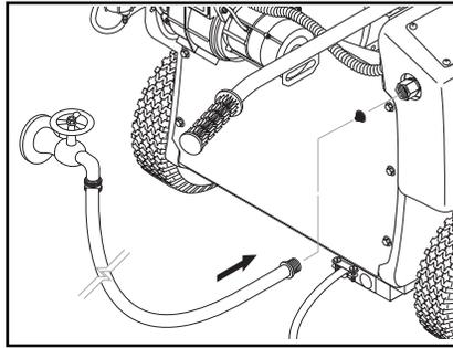
**STEP 2:** Water source for machines should be supplied by a 3/4" I.D. garden hose with a city water pressure of not less than 30 PSI. If the water supply is inadequate, or if the garden hose is kinked, the machine will run very rough and the burner will not fire.
